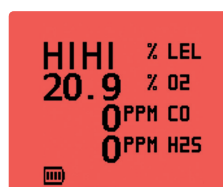
Red display in alarm conditions
